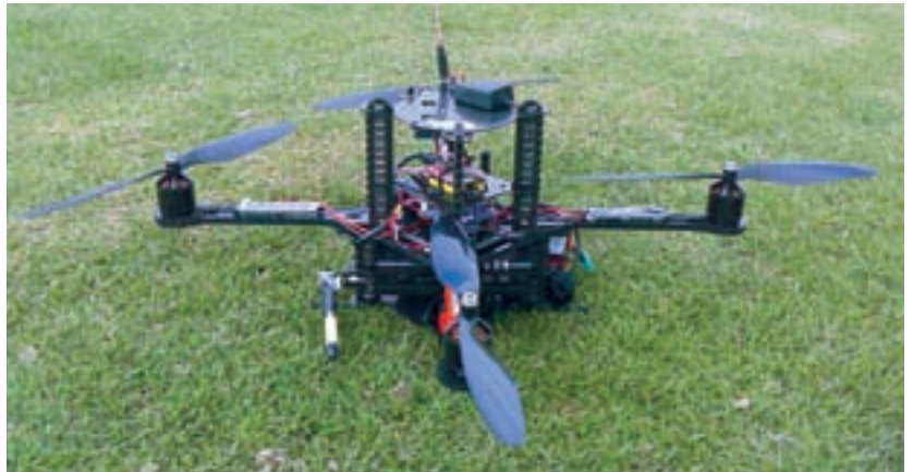
Figure 1: quad-rotor UAV equipped with sensors and Cognitive Radio. Figure 2 (opposite): UAV bridging wireless communications.
