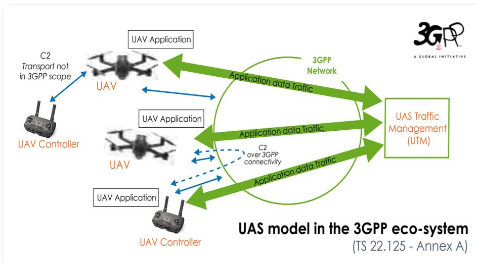
components to establish the necessary connectivity between each other and UAS Traffic Management (UTM) – for both line of sight connectivity and non-line of sight connectivity, and on the detection and reporting of unauthorized UAVs towards the UTM.
